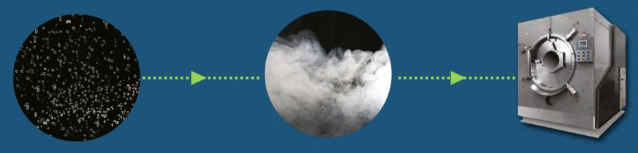
Air, water and chemicals are introduced into the ultra low liquor ratio machine, creating a mixture of nano-bubbles and moist air.
